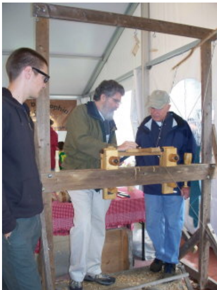
Spring Pole lathe demonstration by Richard Montague
